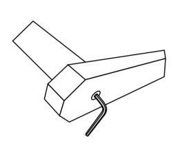
1. Undo one **L** bolt on both poles on the right side of the chair using a 6mm hex key.
